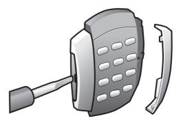
To release Security Caps push a screwdriver into slots on the side and pull forward.
